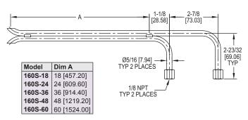
The Series 160S "S" Type Stainless Steel Pitot Tubes are designed specifically for flow measurement of dirty, particulate laden air or gas streams typical in smoke stack and other environmental testing. Total and static pressure tubes are precisely aligned and welded together every 6 inches for maximum accuracy, strength, and long term durability. Permanent mount (PM) models include a 1" welded stainless steel sleeve and adjustable compression fitting with 1" MNPT mounting threads.
