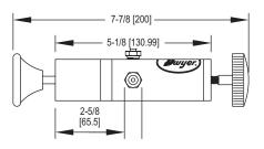
The Model A-396A Calibration Pump serves as pressure source to calibrate gages and transmitters or to set pressure switches. Use with manometer or other pressure standard. Includes volume adjuster enabling fine pressure control and bleed valve. Generates pressures from a fraction of an in w.c. to 72 psig (5 bar). Includes barbed fitting, tee connector and three 36" lengths of vinyl tubing.
